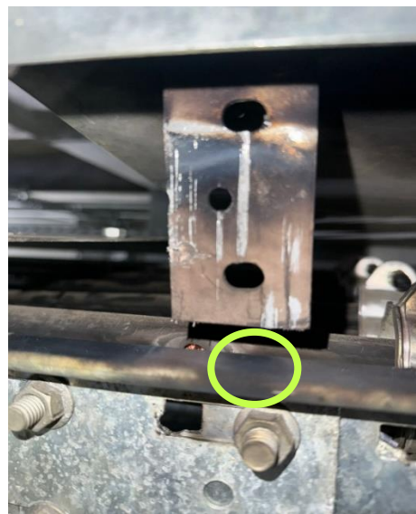
Damaged cable with live conductor showing
